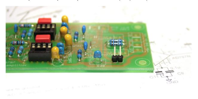
Prepare connectors. Combine connector - groove and comb let us get a single 5-pin block.
