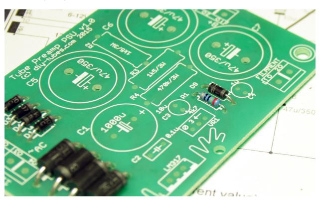
Solder resistors R2-R4 (they're 3W on PCB), the kit includes 2W resistors.
