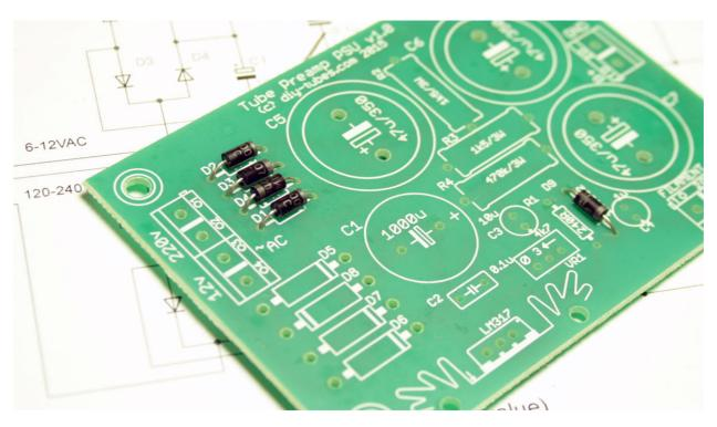
Solder filament diodes (UF5408). You can use other types for lower current. Pay attention to how the diodes are oriented on the board.
