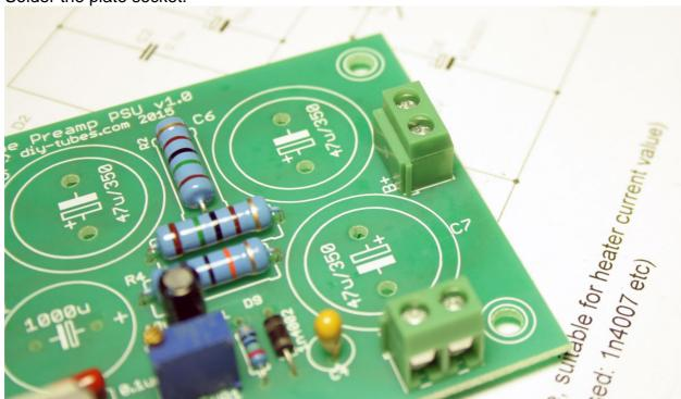
Solder C1 (1000u/50v). Pay attention to how the capacitor is oriented on the board. The negative pole is marked on the body of the condenser with light stripe.
