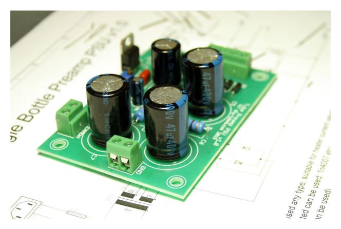
After we finished the installation, it is necessary to connect the secondary winding of the transformer to the appropriate connectors power supply and set the required voltages with trimmer potentiometer and changing R2-R4 (if needed).
