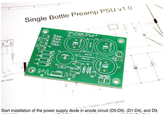
Start installation of the power supply diode in anode circuit (D5-D9). (D1-D4), and D9. (1N4002 on board, use here UF4007 from the kit). You can use 1N4007 (D1-D4) and 1N4002 as D9. Pay attention to how the diodes are oriented on the board.
