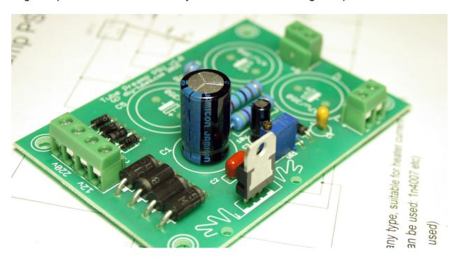
Plate filter capacitors – 3pcs 47u/400v (C5-C7). Other types (voltage and capacitance) can be used here. Pay attention to how the capacitor is oriented on the board. The negative pole is marked on the body of the condenser with light stripe.
