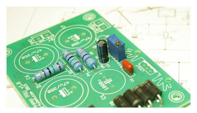
Solder tantalum capacitor. You can use 1u electrolytic capacitor here. Pay attention to how the capacitor is oriented on the board. Plus is marked on body.
