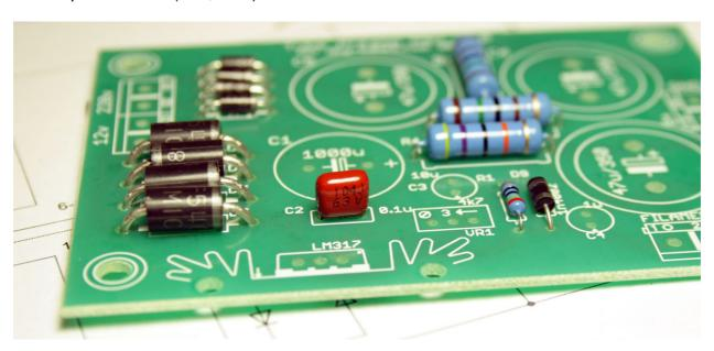
Solder C3 (10u63v). Pay attention to how the capacitor is oriented on the board.
